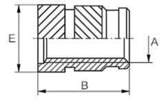
Female thread A = M5 Length B = 8.2 Min distance to edge = 2.7 Outer diameter E = 7.0 Recommended bore diameter W +0.1 = 6.4
